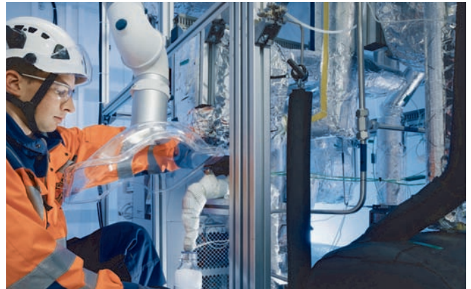
VTT's mobile synthesis unit MOBSU for bench-scale process development. (Photo by COMSYN-project)
