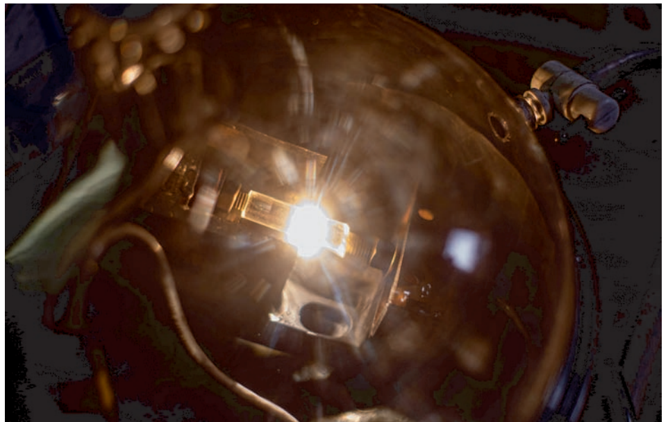
Carbon black powder turns into graphene in a burst of light and heat through a technique developed at Rice University. Flash graphene turns any carbon source into the valuable 2D material in 10 milliseconds. Photo: Jeff Fitlow
