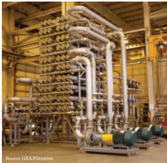
FIGURE 3. Crossflow filtration, microfiltration, nanofiltration, ultrafiltration and reverse osmosis plants can all be placed on modular skids
